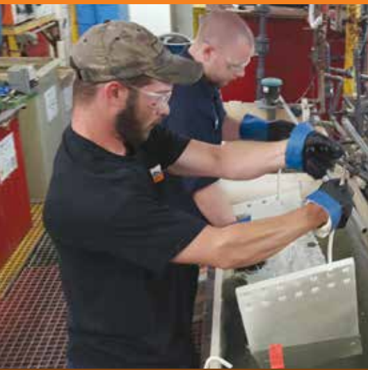
A high-voltage bus bar for an electrical generation plant being silver plated
