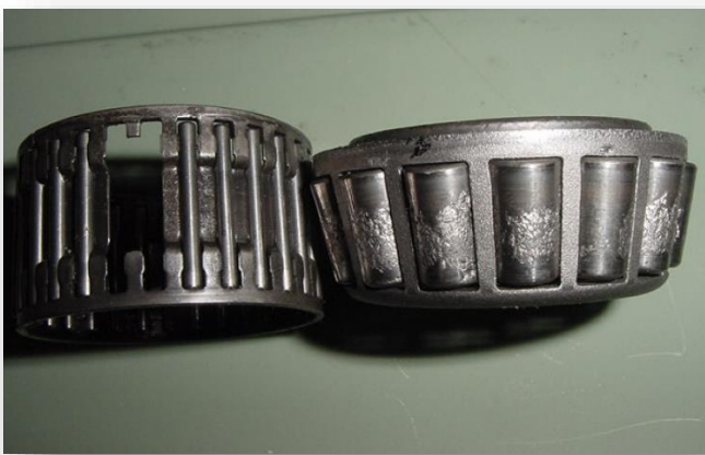
Fretting or galling prevented with AnoLube 9650
