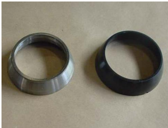
Before (left) and after (right) AnoBlack SS finishing
