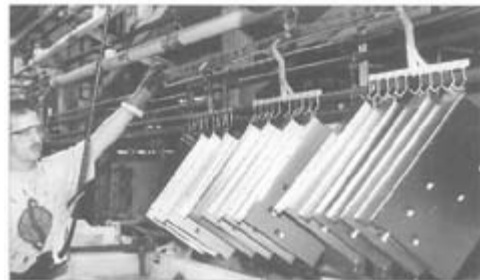
Parts can be closely racked in EN processing, making it cost-effective for high-volume runs.
