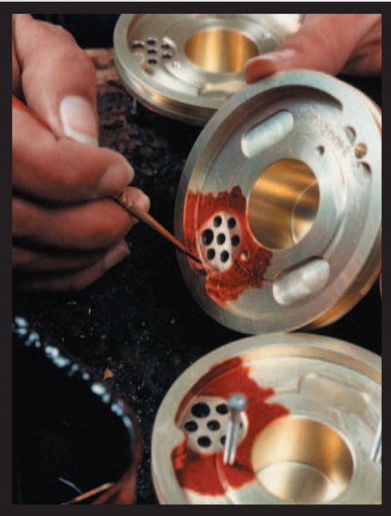
In preparation for actual plating, Anoplate provides special masking, racking, cleaning, stripping and blasting services.
