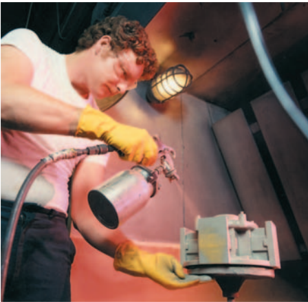
While we do some painting, much of what we apply are dry film lubricants. We have the ability to apply many types of mil-spec paints as well as Molykote®, Everlube®, Teflon® and Xylan coatings.
