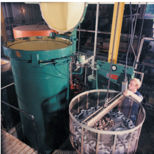
With a chamber measuring 48 inches in diameter and 109 inches deep, Anoplate's vacuum impregnation vessel is one of the largest in North America.
