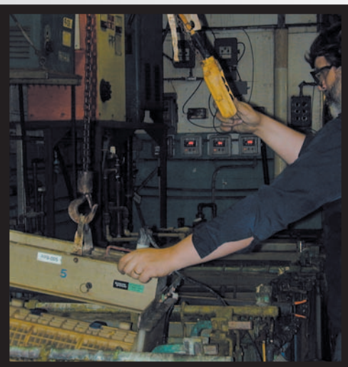
Barrel plating equipment permits economical bulk processing of small to medium-sized parts.
