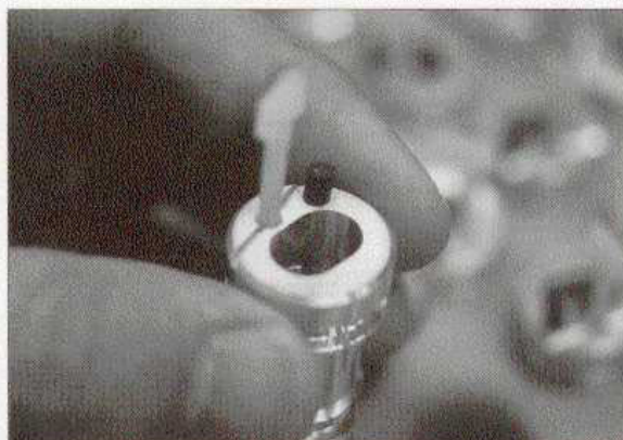
■ This optical component for the medical industry is hard-anodized outside for durability, and Type II black-anodized inside to minimize reflection.
